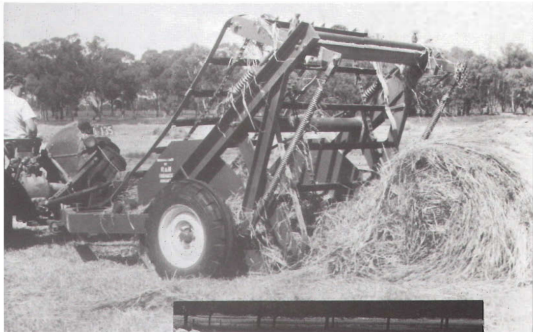
The Econ Roller hay collector enables a greater amount of hay to be "bundled" as a single unit. A comparison between the Econ and conventional hay bales is shown (inset).
