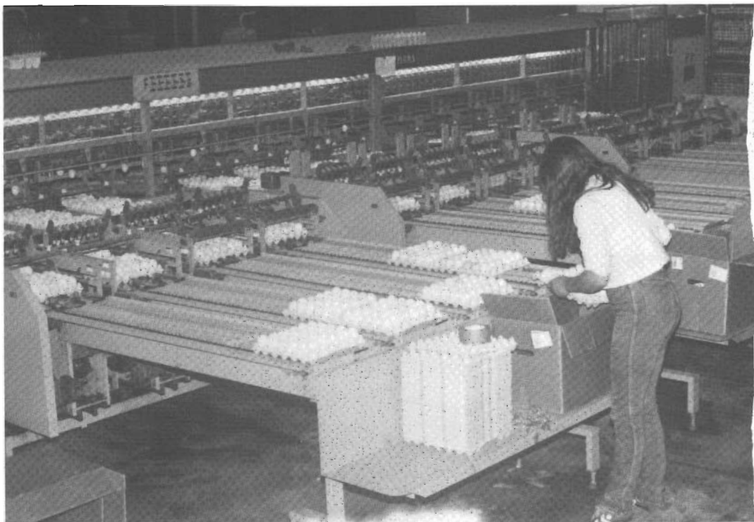
This egg grading equipment is capable of handling 24,000 eggs per hour.
