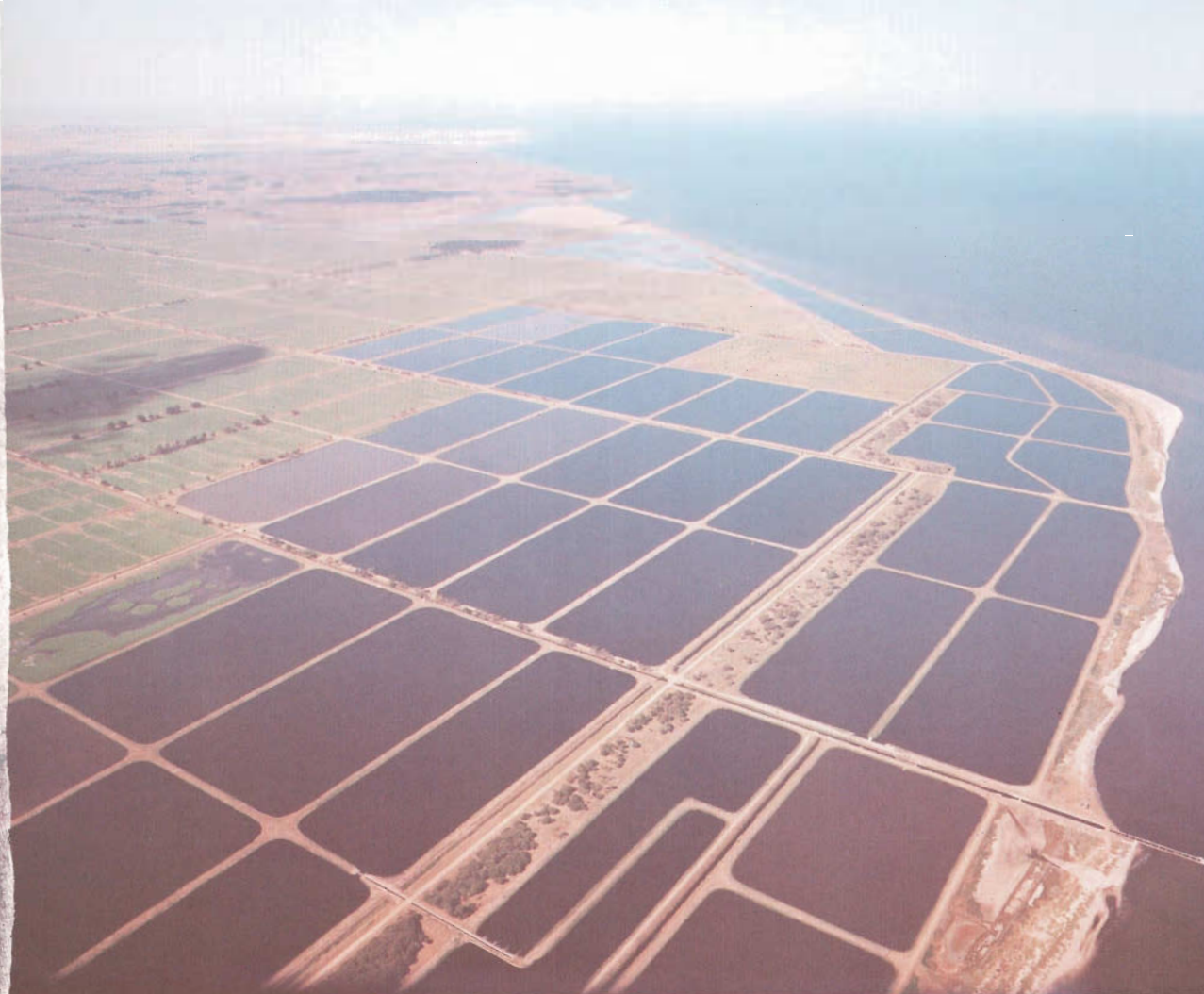
Aerial view of the Werribee Farm showing lagoon treatment of wastewater on the edge of Port Phillip Bay.
