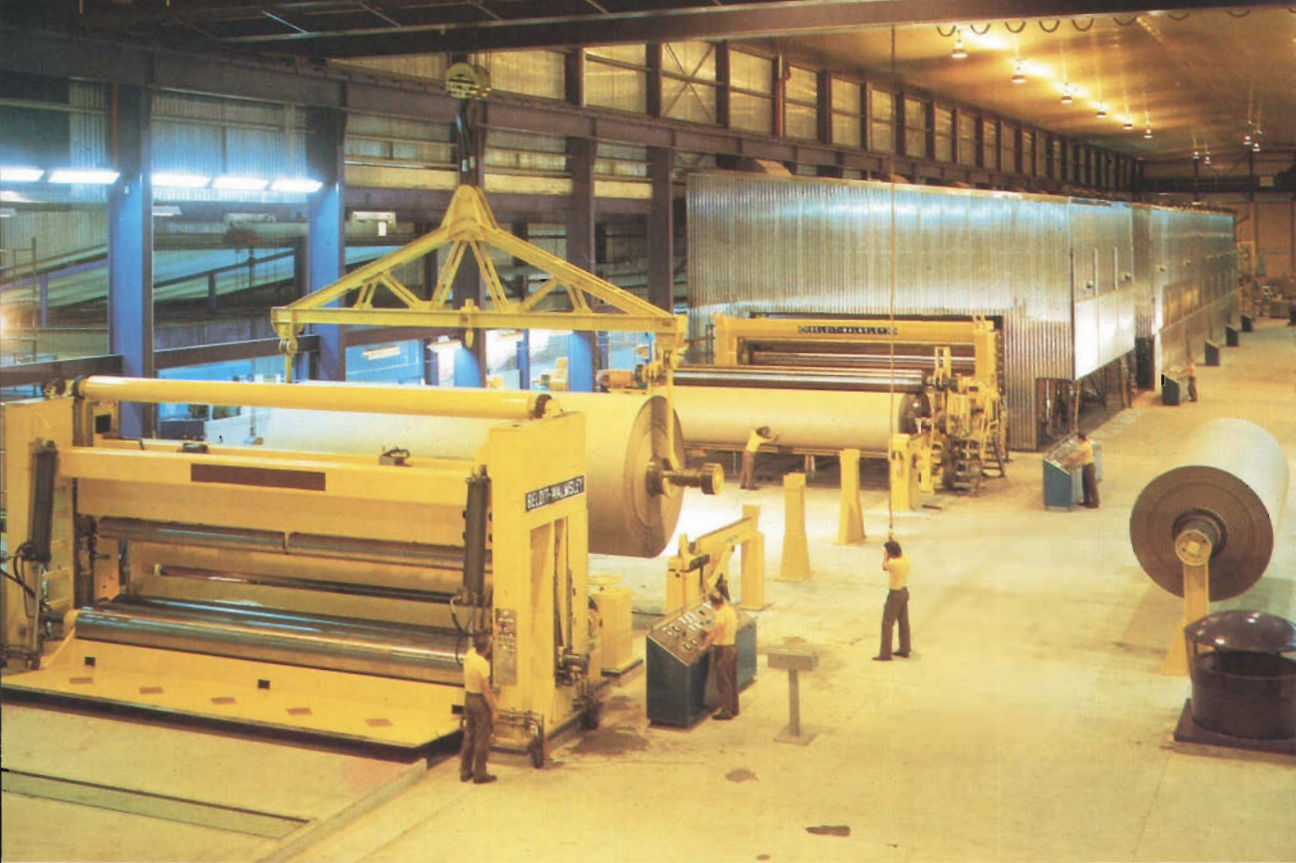
This paper manufacturing machine, Maryvale No. 4, has a capacity of 175,000 tonnes per year.
